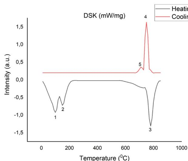
**Figure 1.** Differential scanning calorimetry method for the BaBrI system: peaks 1 and 2, associated with a phase transition of water leaving the raw material; peak 3, melting temperature of BaBrI, 781 °C; peak 4, crystallization process at 754.5 °C; peak 5, phase transition associated with a change in the type of lattice at 730 °C.
