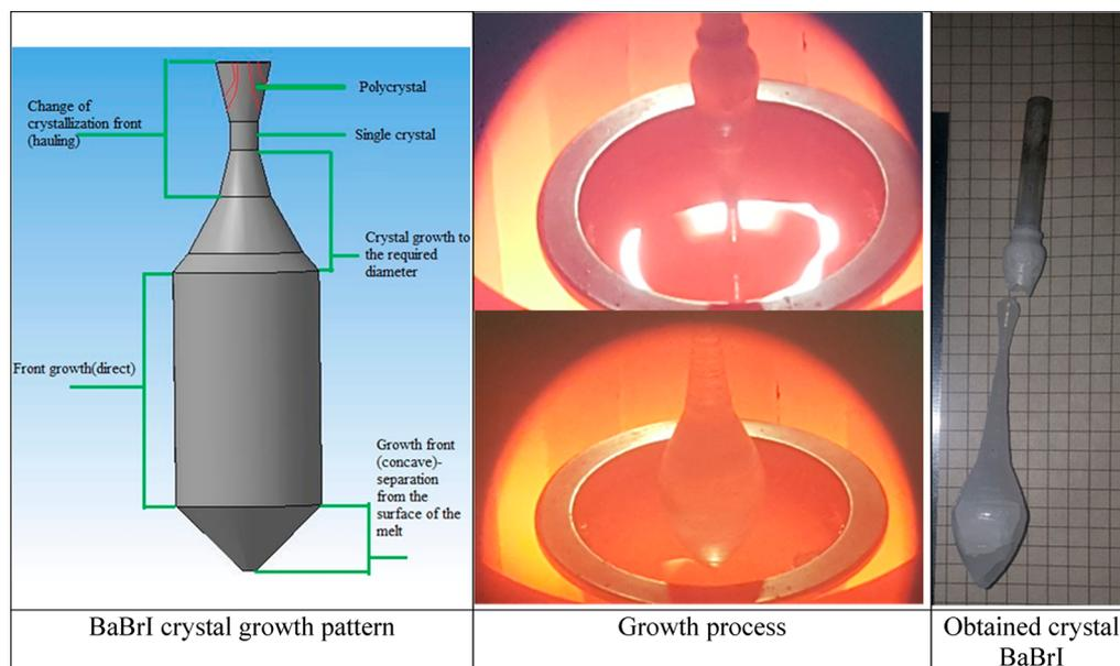
**Figure 4.** Structure of BaBrI crystals: polycrystal, formed from a supercooled melt; single crystal, formed by changing the surface temperature of the melt; growth of a single crystal (permanent form), the ratio of the growth rate and the surface temperature of the melt is maintained; separation from the surface, temperature increase (crystal decrease) and movement to the cooling area.
