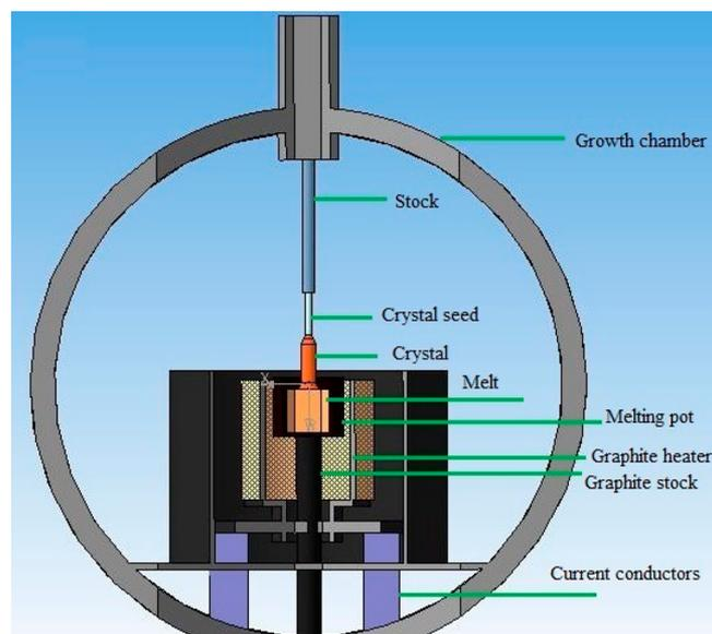
**Figure 2.** Scheme of the apparatus for crystal growth.
