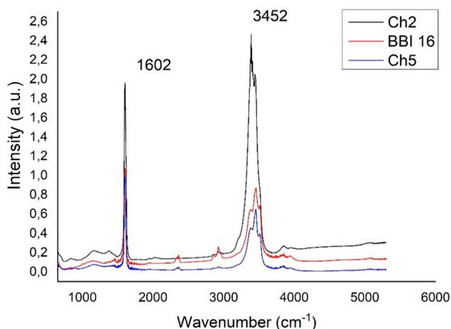
**Figure 6.** Fourier Transform Infrared (FTIR) absorption spectra of BaBrI crystals.
