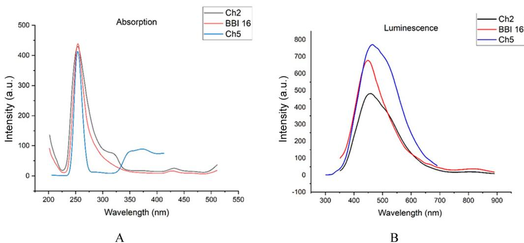
**Figure 5.** Excitation (A) and luminescence (B) spectra of BaBrI crystals.
