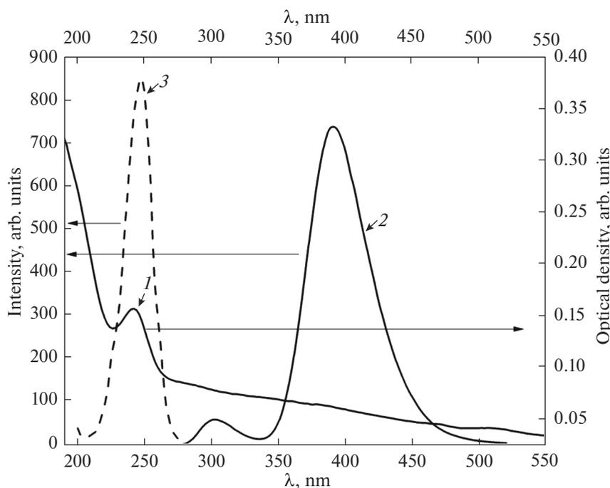
**Fig. 1.** Absorption spectra (1), photoluminescence (2) ( $\lambda_{\text{excitation}}$ , 240 nm) and excitation (3) ( $\lambda_{\text{lum}}$ , 302 nm) of quartz glass, measured at room temperature.
