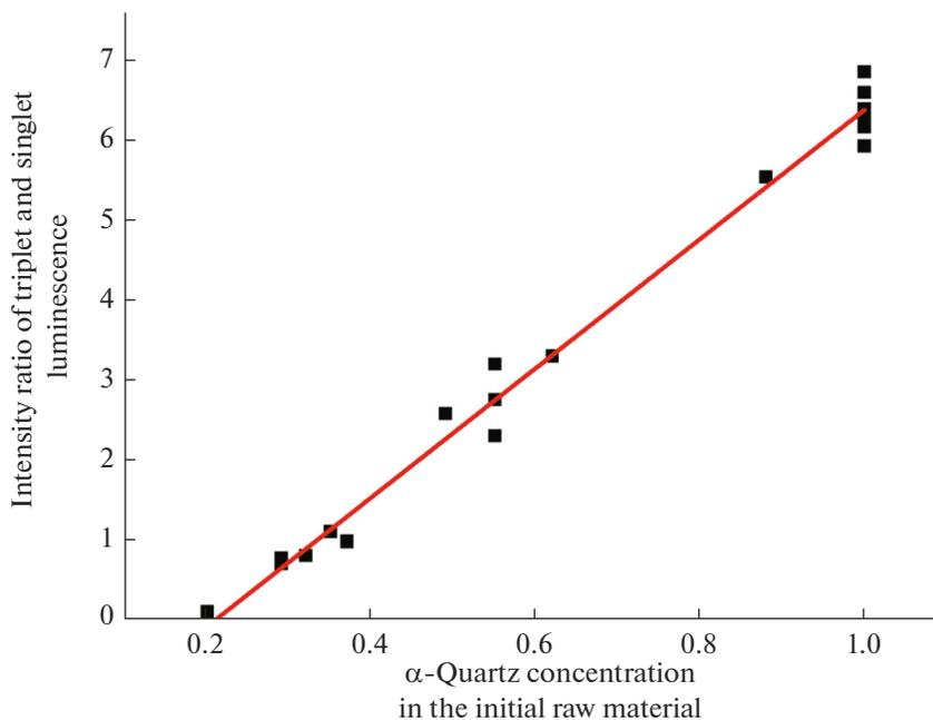
**Fig. 3.** Dependence of the intensity ratio of the triplet and singlet luminescence of Ge-ODCs(II) on the content of the  $\alpha$ -quartz phase in the feedstock.
