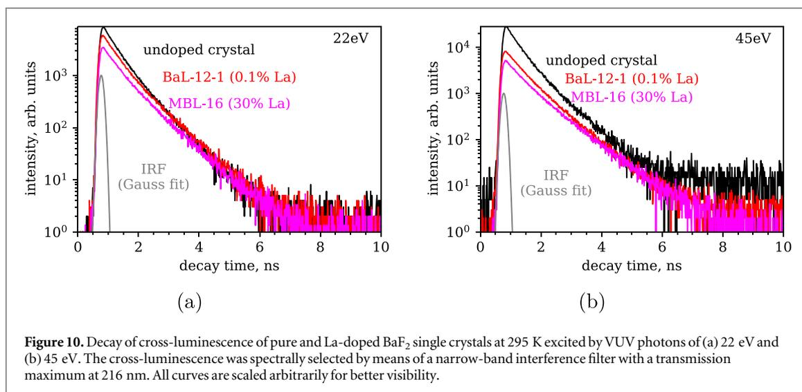
**Figure 10.** Decay of cross-luminescence of pure and La-doped BaF<sub>2</sub> single crystals at 295 K excited by VUV photons of (a) 22 eV and (b) 45 eV. The cross-luminescence was spectrally selected by means of a narrow-band interference filter with a transmission maximum at 216 nm. All curves are scaled arbitrarily for better visibility.
