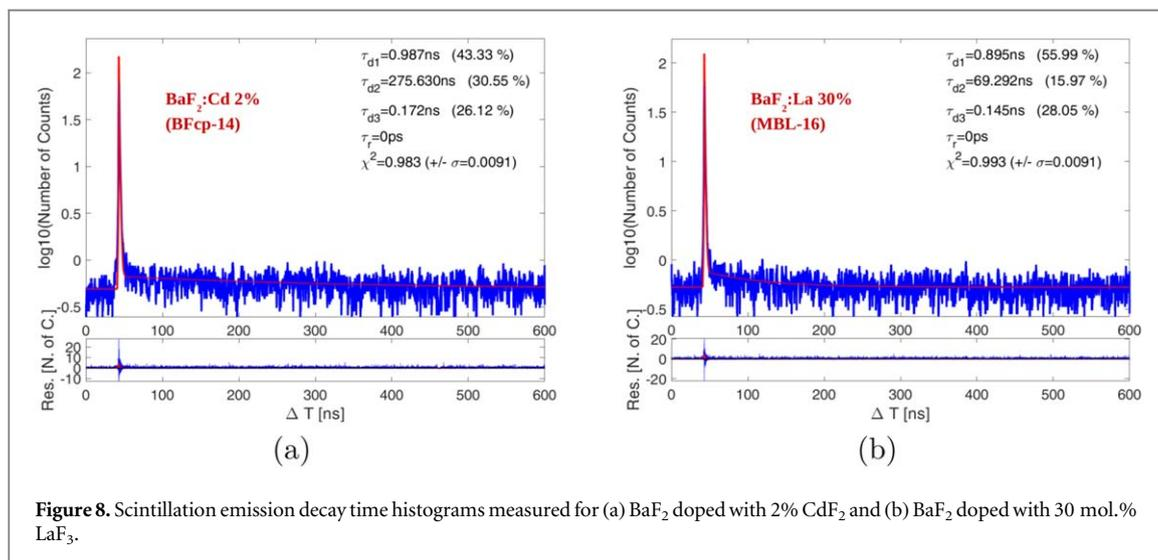
**Figure 8.** Scintillation emission decay time histograms measured for (a) BaF<sub>2</sub> doped with 2% CdF<sub>2</sub> and (b) BaF<sub>2</sub> doped with 30 mol.% LaF<sub>3</sub>.
