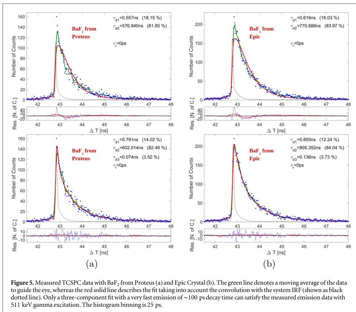
**Figure 5.** Measured TCSPC data with  $\text{BaF}_2$  from Proteus (a) and Epic Crystal (b). The green line denotes a moving average of the data to guide the eye, whereas the red solid line describes the fit taking into account the convolution with the system IRF (shown as black dotted line). Only a three-component fit with a very fast emission of  $\sim 100$  ps decay time can satisfy the measured emission data with 511 keV gamma excitation. The histogram binning is 25 ps.
