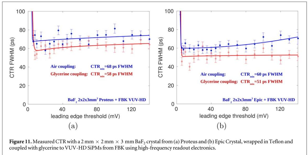
**Figure 11.** Measured CTR with a  $2\text{ mm} \times 2\text{ mm} \times 3\text{ mm}$   $\text{BaF}_2$  crystal from (a) Proteus and (b) Epic Crystal, wrapped in Teflon and coupled with glycerine to VUV-HD SiPMs from FBK using high-frequency readout electronics.
