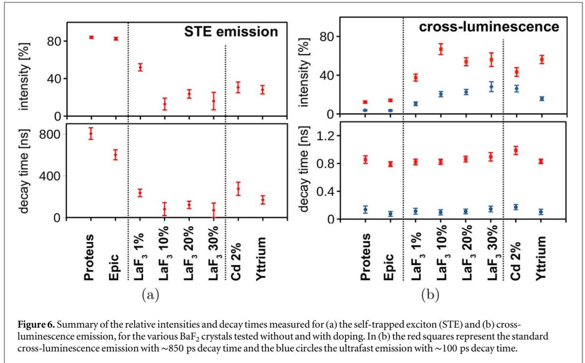
**Table 5.** The scintillation time characteristics of BaF<sub>2</sub> compared for samples with different doping, suppressing the slowest decay time component ( $\tau_{d3}$ ). Every doping tested successfully suppresses the slow 800 ns STE emission. Errors are given in  $\pm 1\sigma$ , meaning a confidence interval of 68%.
