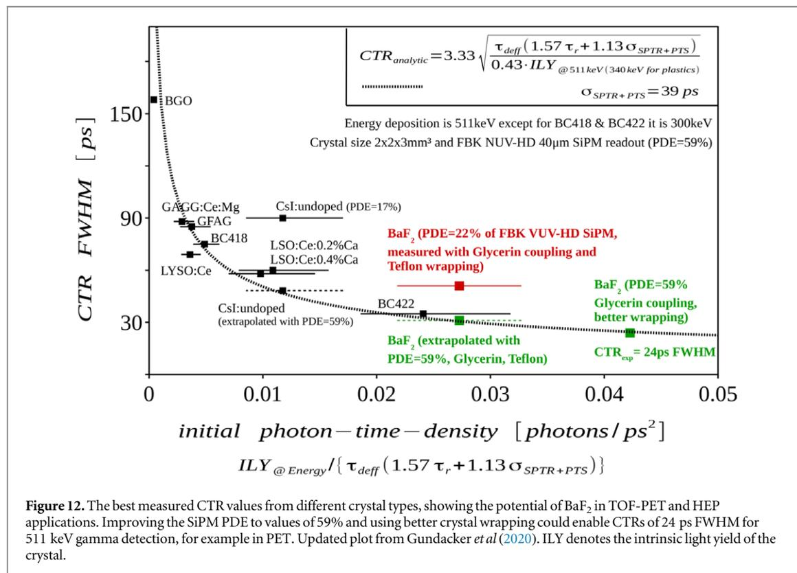
at 420 nm. In view of the ultrafast, almost prompt, emission in BaF<sub>2</sub> with decay times below 100 ps, the SPTR gains a special importance, as was shown in Gundacker *et al* (2016). Hence, improving the SPTR of the VUV-SiPM opens an additional route to push the CTR limits with BaF<sub>2</sub> even further (Acerbi and Gundacker 2019, Lecoq *et al* 2020).
