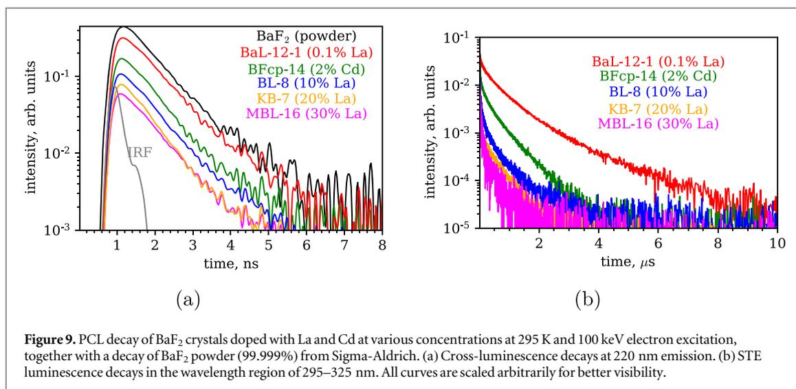
**Figure 9.** PCL decay of BaF<sub>2</sub> crystals doped with La and Cd at various concentrations at 295 K and 100 keV electron excitation, together with a decay of BaF<sub>2</sub> powder (99.999%) from Sigma-Aldrich. (a) Cross-luminescence decays at 220 nm emission. (b) STE luminescence decays in the wavelength region of 295–325 nm. All curves are scaled arbitrarily for better visibility.
