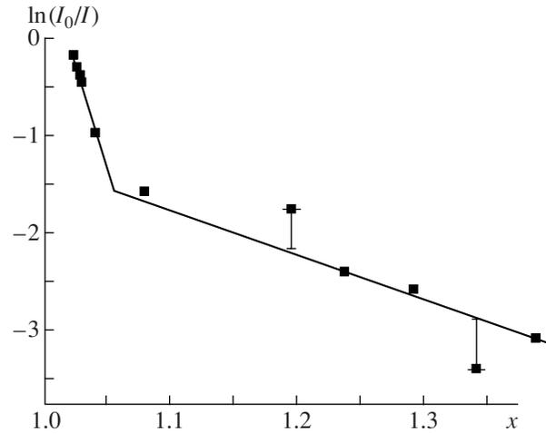
**Fig. 2.** Dependence of  $\ln(I_0/I)$  on the variable  $X = 1 + 2\pi^2 T^2 / 3\theta_D^2$  for the 839.5-nm ZPL; the sample is  $\gamma$ -irradiated ( $2.58 \times 10^4$  C/kg) and optically bleached in the quantron of a KVANT-17 laser ( $n = 10$  pulses);  $\theta_D = 275$  K.
