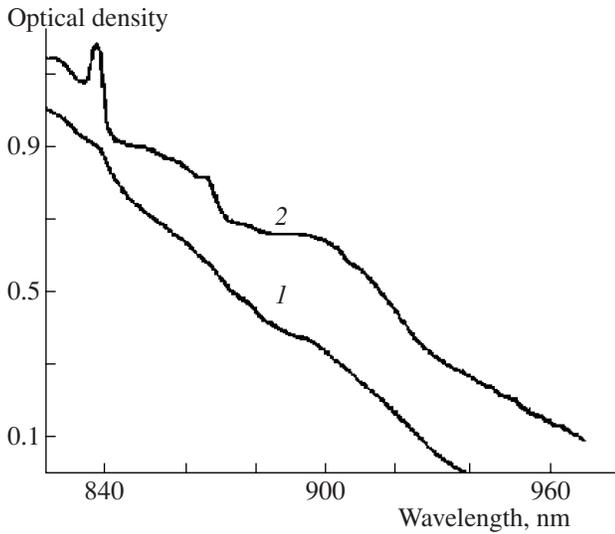
**Fig. 1.** Absorption spectra of a  $\gamma$ -irradiated NaCl crystal (dose  $2.58 \times 10^4$  C/kg), recorded at temperatures  $T = (1)$  80 and  $(2)$  17 K.
