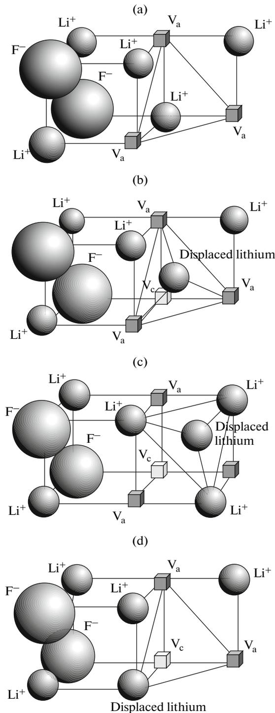
**Fig. 1.** Schematic of the studied spatial configurations of precolloidal centers in a superlattice: (a) base configuration; (b) the lithium nearest the plane of anionic vacancies is displaced to the geometrical center of the (111) plane; (c) the lithium nearest the plane of anionic vacancies is displaced to the geometric center of cations; (d) the lithium nearest the plane of anionic vacancies is displaced to anionic vacancies.
