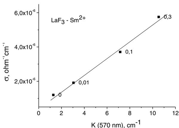
Fig.4. Conductivity of  $\text{LaF}_3\text{-Sm}^{2+}$  samples against of absorption coefficient of absorption band at 570 nm at room temperature. Concentrations of doped  $\text{SmF}_3$  are shown near experimental points.
