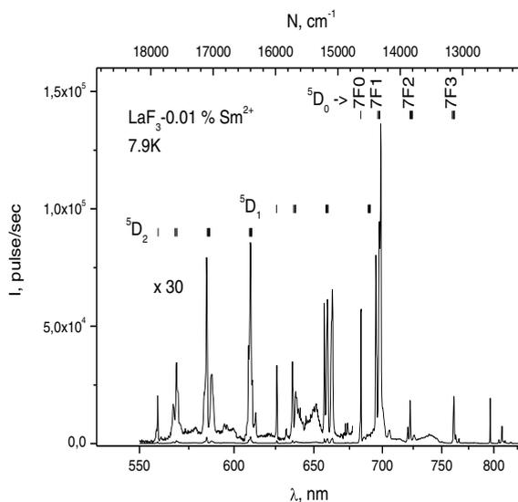
Fig.2. Emission spectra of  $\text{LaF}_3\text{-0.01 \% Sm}^{2+}$  crystal at temperature 7.9 K. Left part of spectrum are increased by 30 times. Transitions from  $^5D_j$  to  $^7F_j$  are shown at the top of graph
