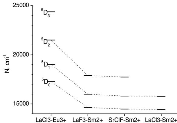
Fig.3. Scheme of  $^5D_j$  energy levels of isoelectronic  $\text{Eu}^{3+}$  in  $\text{LaCl}_3$  (Kumar et al. 1977),  $\text{Sm}^{2+}$  in  $\text{SrClF}$  (Grenet et al.1980),  $\text{Sm}^{2+}$  in  $\text{LaCl}_3$  (Dieke et al.1962) and  $\text{Sm}^{2+}$  in  $\text{LaF}_3$ . In  $\text{Sm}^{2+}$  ion the energies of levels reduced by near 20% against that in  $\text{Eu}^{3+}$ .
