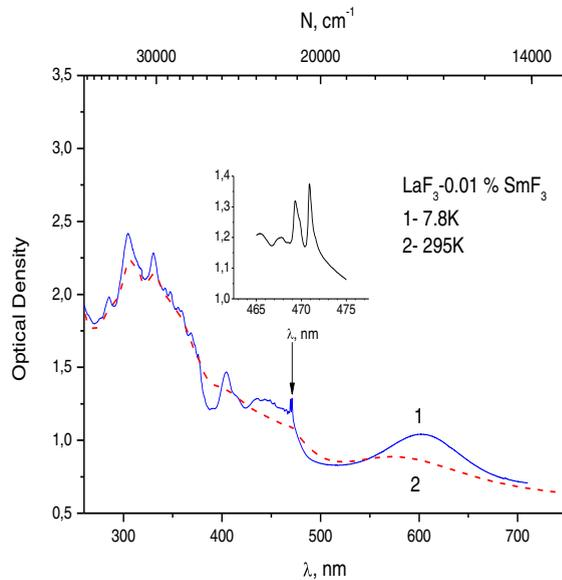
Fig.1. Absorption spectra of  $LaF_3$ -0.01 %  $Sm^{2+}$  (thickness 2.5mm) at temperature 7 K (curve 1) and 295 K (curve 2). The inset in the graph displays the fine structure of spectrum. No absorption bands were observed in  $LaF_3$ -0.01 %  $Sm^{3+}$  samples.
