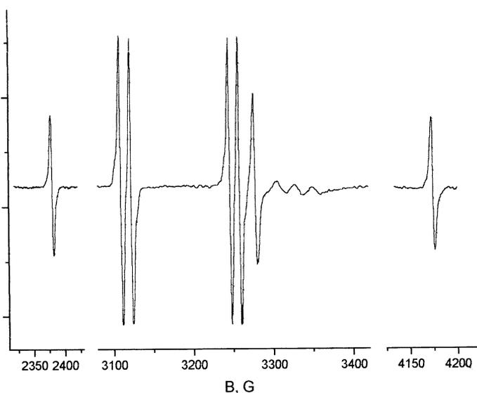
FIGURE 2 EPR spectrum of pure BaF<sub>2</sub> crystal after x-irradiation at 80 K, B || (100).
