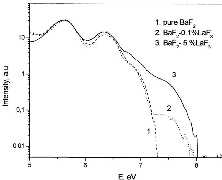
FIGURE 3 X-ray excited luminescence spectra at 80 K of La-doped  $\text{BaF}_2$  crystals.
