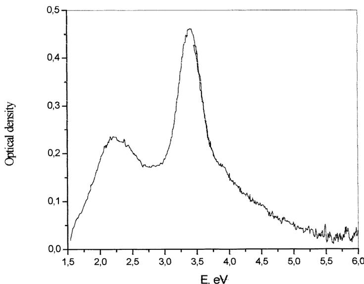
FIGURE 1 Optical absorption of pure  $\text{BaF}_2$  crystal after X-irradiation at 80 K.
