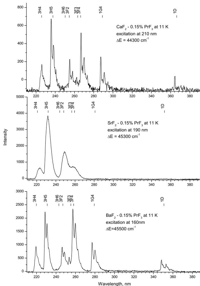
**Figure 1.** Emission spectra of  $\text{Pr}^{3+}$  5d-4f transitions in  $\text{CaF}_2$ ,  $\text{SrF}_2$ ,  $\text{BaF}_2$  crystals doped by 0.15 molar % of  $\text{PrF}_3$ . Positions of each line due to the transitions from the lowest 5d levels to individual 4f levels are shown at the top of each plot.
