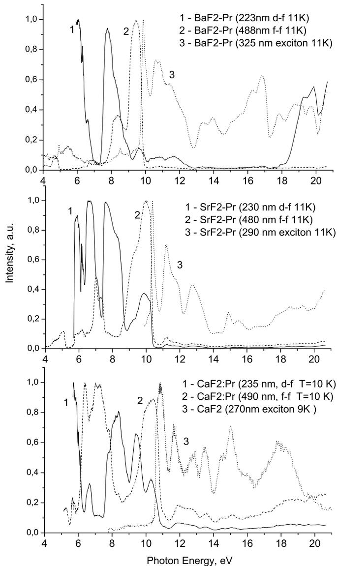
**Figure 3.** Excitation spectra of Pr 5d-4f and 4f-4f emission bands as well as exciton emission of CaF<sub>2</sub>, SrF<sub>2</sub>, BaF<sub>2</sub> crystals doped by 0.15 molar % of PrF<sub>3</sub>.
