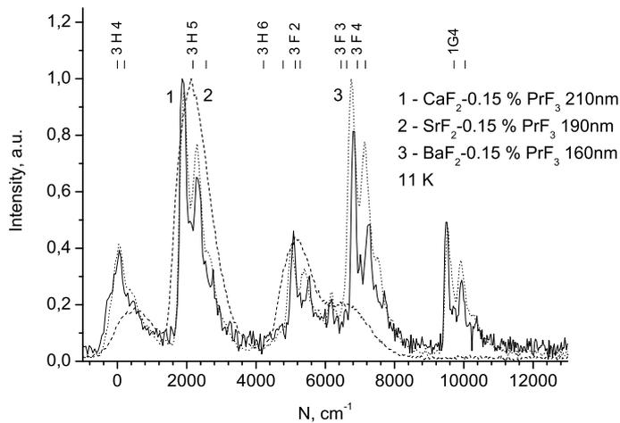
**Figure 2.** Comparison of the shapes of the emission spectra of  $\text{Pr}^{3+}$  5d-4f transitions in  $\text{CaF}_2$ ,  $\text{SrF}_2$ ,  $\text{BaF}_2$ . The spectra are normalized for the  $^3\text{H}_5$  line intensities, while the origin of the wave number scale is placed at the  $^3\text{H}_4$  line.
