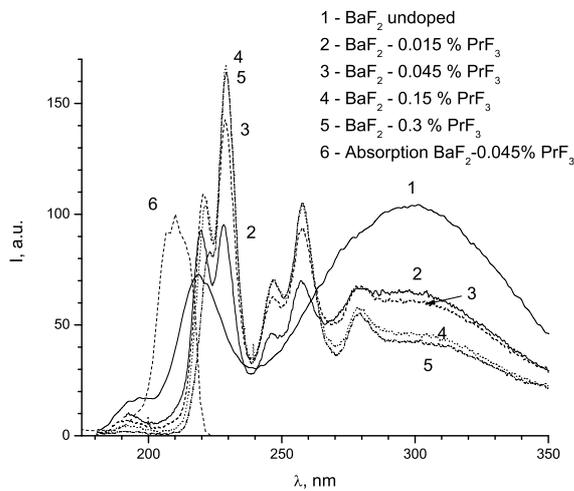
**Figure 4.** Emission spectra of undoped BaF<sub>2</sub> (curve 1) and BaF<sub>2</sub>-PrF<sub>3</sub> (curves 2-5) measured under x-ray excitation at room temperature. Absorption spectrum of BaF<sub>2</sub>-0.045 % PrF<sub>3</sub> in arbitrary units is added for comparison (curve 6).
