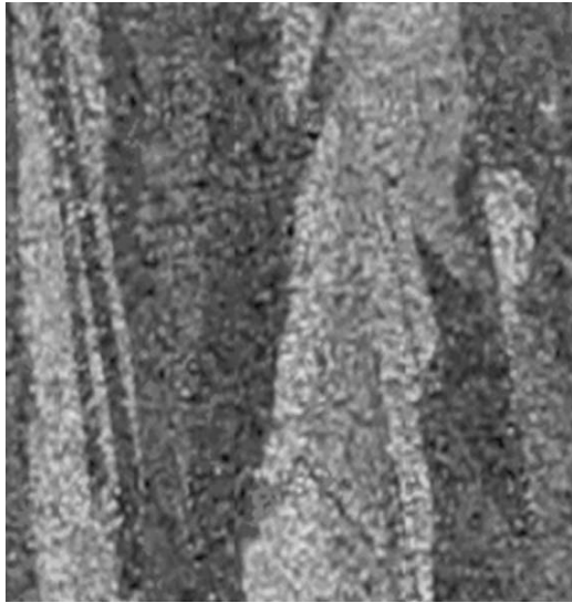
Fig. 1. Image of a typical polycrystalline silicon sample (fragment with dimensions 1.0 \times 1.0 cm).
