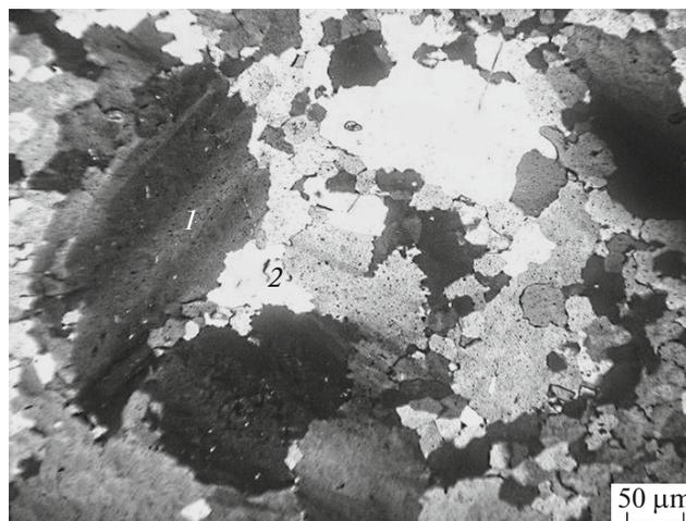
Fig. 2. Quartz generations in superquartzite: the (1) first (relict) and (2) second generations.
