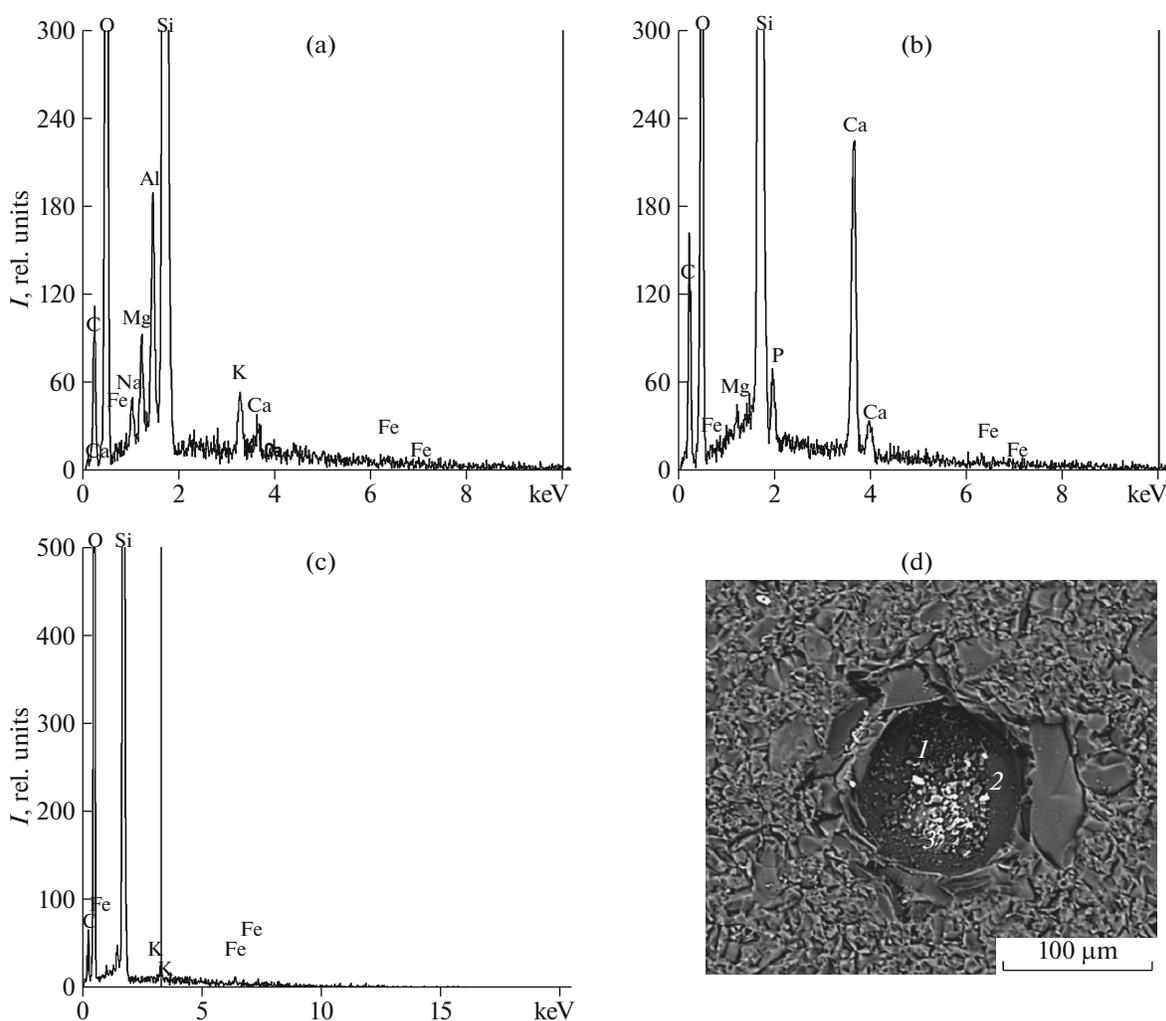
**Fig. 5.** (a–c) EDS spectra characterizing the elemental composition of specific inclusions, which are indicated in the (d) back-scattered electron image of the surface of the central part of the glass plate obtained from superquartzite.
