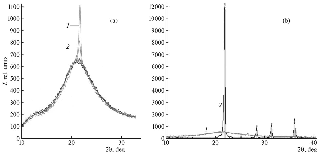
Fig. 4. Fragments of diffraction patterns: (a) quartz glass after plate annealing at (1) 1150°C and (2) 1200°C and (b) (1) ground quartz glass sample, previously annealed at 1200°C, and (2) ground glass sample after repeated annealing to 1300°C.
