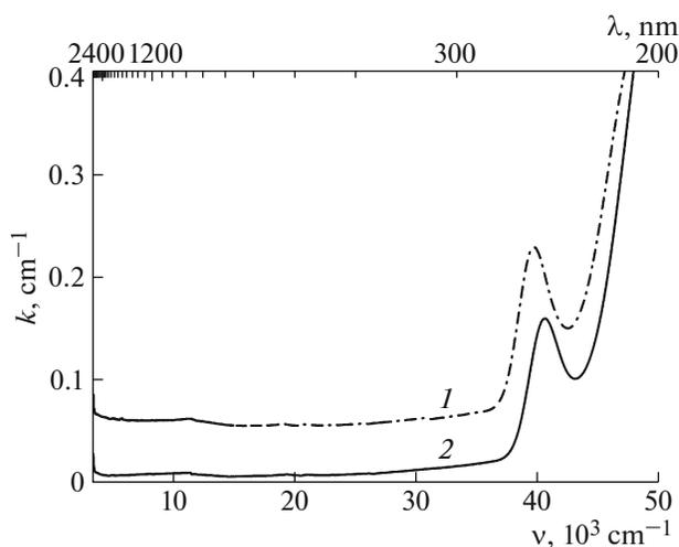
Fig. 3. Absorption spectra of the quartz glasses obtained from superquartzite cristobalite grit molten at pressures of (1) 1 and (2) 5 bar.
