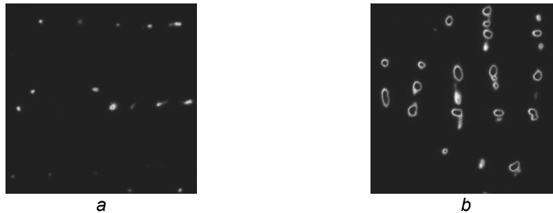
Fig. 2. The transverse distribution of the fluorescence intensity of the color centers formed by laser irradiation (scan area 80 \times 80 \mu\text{m} ): a – energy radiation 13,75 mJ (25 counts); b – the energy of radiation 550 mJ (1000 pulses).
