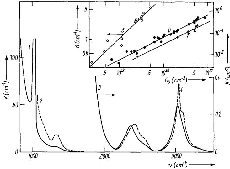
Fig. 2. Infrared absorption spectra of  $\text{LiF:H}^-$  crystals with different concentrations of U-centres; (1)  $3 \times 10^{19}$ , (2)  $10^{20}$ , (3)  $5 \times 10^{20} \text{ cm}^{-3}$  at 295 K, and (4)  $5 \times 10^{20} \text{ cm}^{-3}$  at 80 K. The variation with the U-centre concentration of the absorption coefficient of the bands at (5) 1320, (6) 3020, and (7)  $2360 \text{ cm}^{-1}$  at 295 K is shown in the inset
