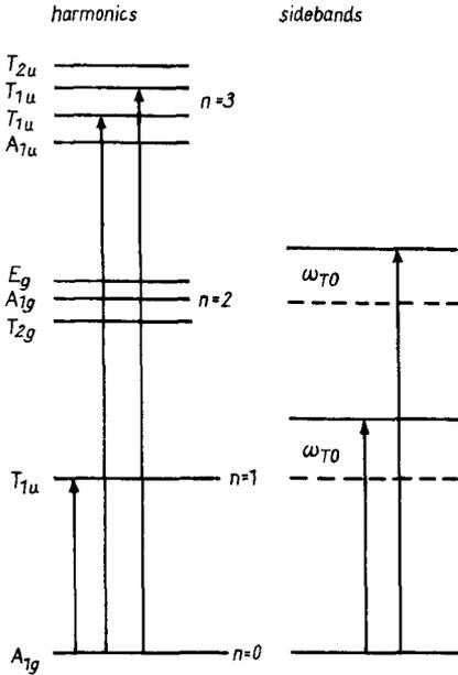
Fig. 1. Schematic representation of the vibrational energy levels of the U-centre in LiF. Observed transitions are indicated by vertical lines
